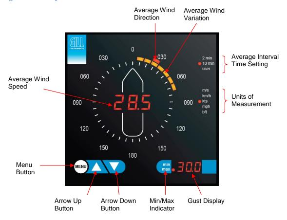
On the front panel of the display there are three push buttons, "MENU" "▲"and "▼". An explanation of front panel button functions is as follows:-
