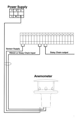
When both the anemometer and display are powered on wind speed data should be read on the 3 digit speed display and direction data indicated by the outer circles of LED's. The information update rate will be once per second.
