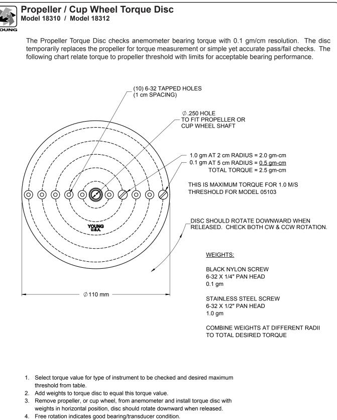
5. Failure to rotate indicates need for service.
