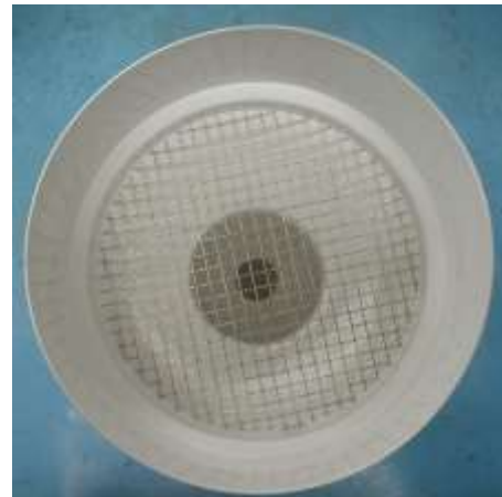
FIGURE 2.7: COLLECTION FUNNEL & ORIFICE SCREENS
