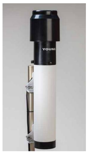
When the column level reaches a maximum of 250 mm (50 mm of precipitation), the chamber automatically empties and the process repeats. Total precipitation can be tracked by a datalogger or recorder.
