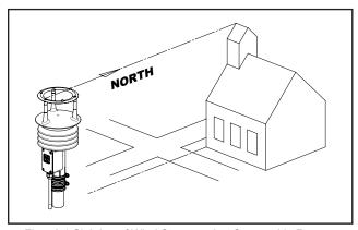
Fig 4.2.1 Sighting of Wind Sensor using Geographic Feature
