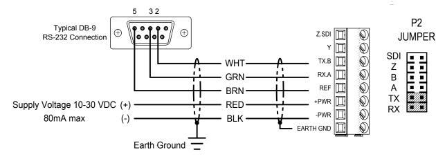
Figure A2: RS-485 / RS-422 SERIAL CONNECTION - FULL DUPLEX
