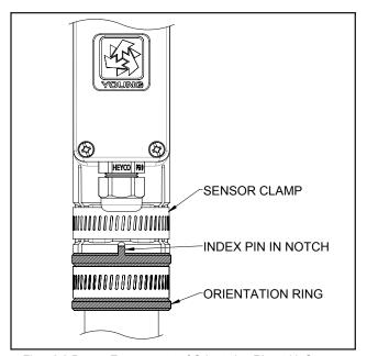
Fig 4.2.2 Proper Engagement of Orientation Ring with Sensor
