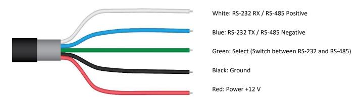
The Green wire should be connected to Ground to enable RS-485 communication, or it should be connected to 12 V power for RS-232 communication. Text for the White and Blue wires above refers to the port that the wires should be connected to.
