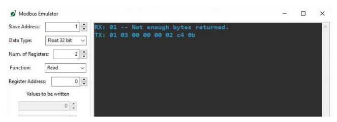
Solutions: [1] Check wiring and protocol [2] Unplug and then plug AC-422 back in.
