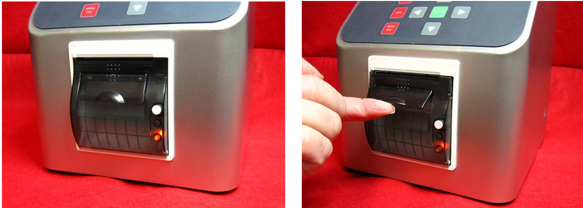
Figure 5 – Open Printer Door
