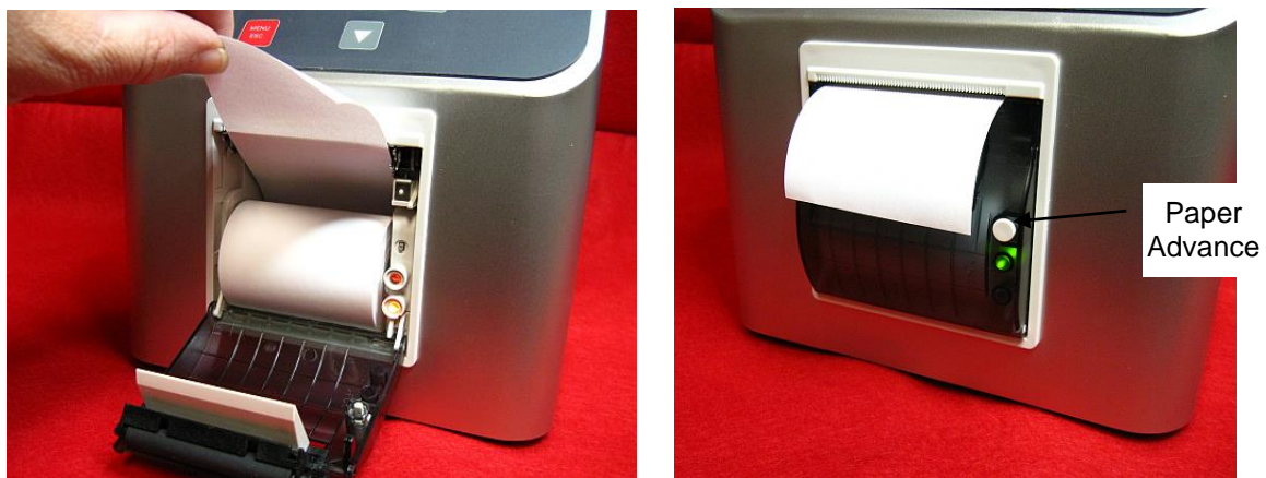
Figure 6 – Install Paper and Close Printer Door
