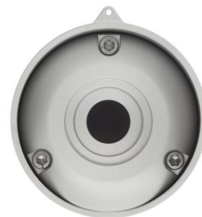
Figure 5 DR30 digital pyrheliometer front view
