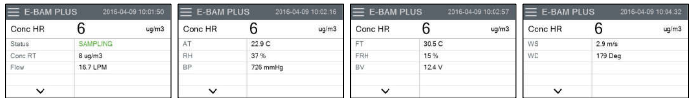
Figure 3-2 The E-BAM PLUS Main Operating Screens
