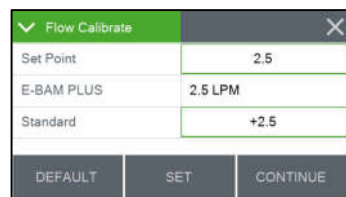
Figure 6-13 Sheath Air Calibration Screens
