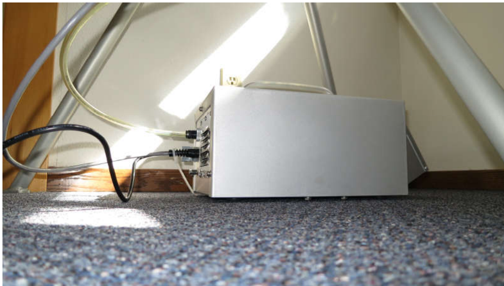
Figure 2-5 Connecting the EX-225 or EX-226 Pump Box
