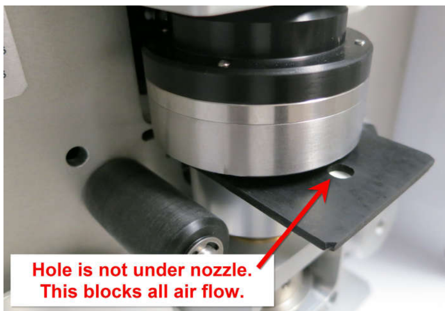
Figure 6-5 Nozzle Sealing Tool Lower System Test Configuration
