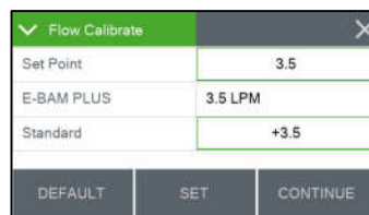
Figure 6-13 Sheath Air Calibration Screens
