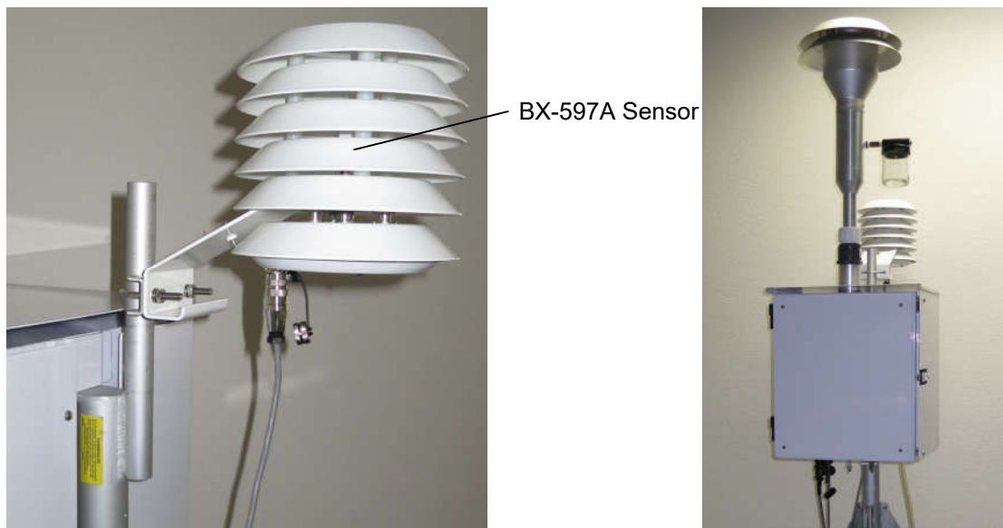
Figure 2-3 Mounting the BX-597A Sensor
