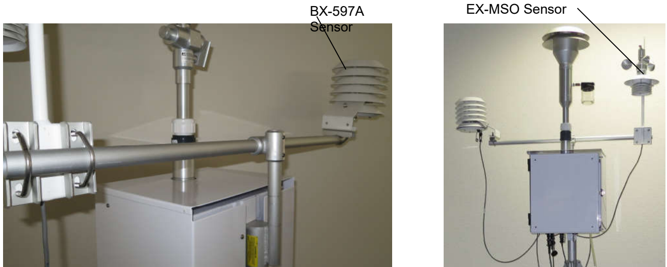
Figure 2-4 Sensor Mounting with an Optional Wind Sensor
