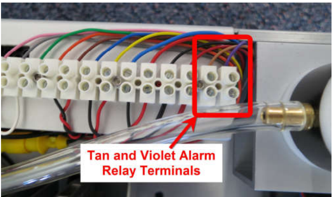
Figure 3-26 AC Pump Box Alarm Relay Terminal Locations
