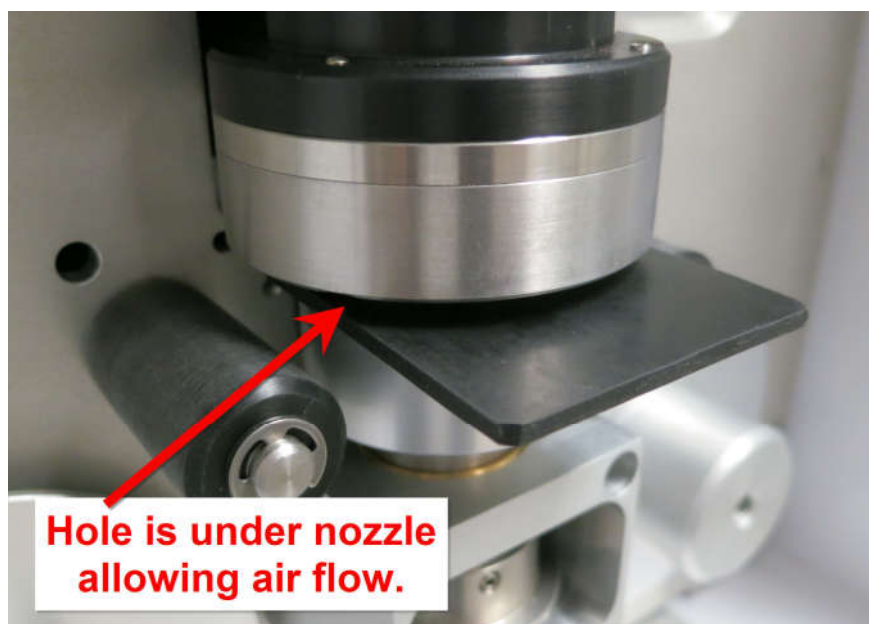
Figure 6-6 Nozzle Sealing Tool Upper System Test Configuration
