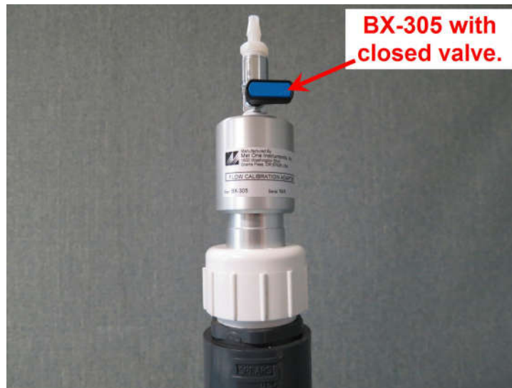
Figure 6-2 BX-305 Installed on Inlet Tube
