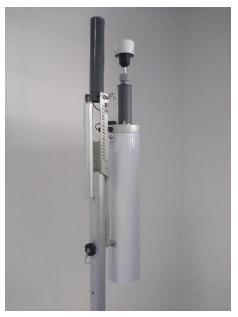
3. Site the tripod on a surface that is as level as possible. The tripod feet may be secured to the ground or mounting surface with bolts, screws, or tent pegs if necessary. Secure the tripod in windy conditions!
