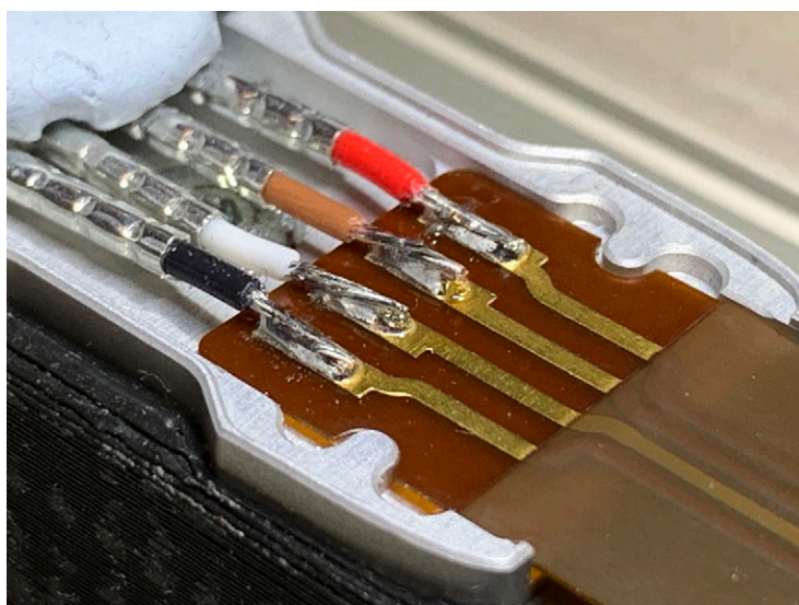
Figure 7.2.2 FHF04 sensor foil with soldered wires.
