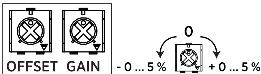
Figure 14 Trimmers for Offset and Gain
