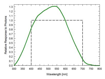
Mean spectral response of four SQ-100X series quantum sensors compared to PPFD weighting function. Spectral response measurements were made at 10 nm increments across a wavelength range of 350 to 800 nm in a monochromator with an attached electric light source. Measured spectral data from each quantum sensor were normalized by the measured spectral response of the monochromator/electric light combination, which was measured with a spectroradiometer.
