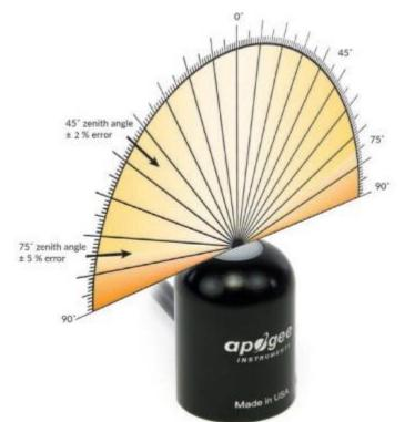
Directional (cosine) response is defined as the measurement error at a specific angle of radiation incidence. Error for Apogee SQ-100X series quantum sensors is approximately  $\pm 2$  % and  $\pm 5$  % at solar zenith angles of 45° and 75°, respectively.
