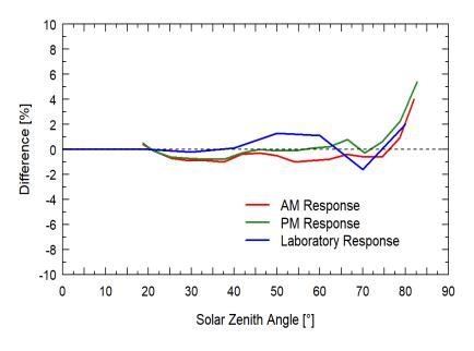
Mean directional (cosine) response of seven apogee MQ-500 series quantum sensors. Directional response measurements were made on the rooftop of the Apogee building in Logan, Utah. Directional response was calculated as the relative difference of MQ-500 quantum sensors from the mean of replicate reference quantum sensors (LI-COR models LI-190 and LI-190R, Kipp & Zonen model PQS 1). Data were also collected in the laboratory using a reference lamp and positioning the sensor at varying angles.
