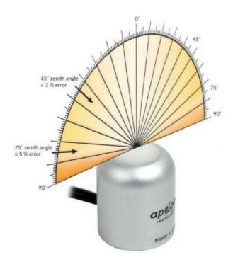
Directional, or cosine, response is defined as the measurement error at a specific angle of radiation incidence. Error for Apogee MQ-600 series ePAR Sensor is approximately  $\pm$  2 % and  $\pm$  5 % at solar zenith angles of 45° and 75°, respectively.
