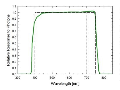
Mean spectral response measurements of four replicate Apogee MQ-600 series ePAR Sensors. Incremental spectral response measurements were made at 10 nm increments across a wavelength range of 370 to 800 nm in a monochromator with an attached electric light source. Measured spectral data from each quantum sensor were refined and normalized by comparing measured spectral response of the monochromator/electric light combination to measured spectral differences from a quantum sensor reference.
