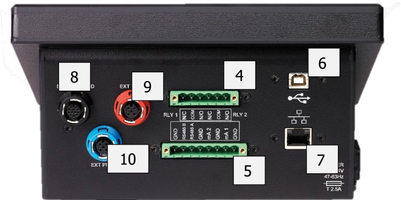
Figure 9 Optidew 401 rear panel
