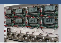
In addition to AMI's superior design every single oxygen sensor manufactured by AMI undergoes a rigorous temperature and performance test before it can be shipped to a customer. Each unit is independently tested for come down time, noise, linearity and diurnal performance while varying temperature.
