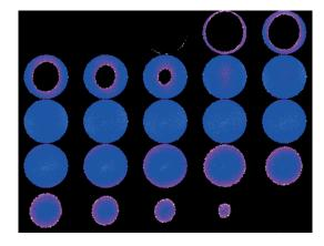
This result shows a LPG-650 laser pulse being stepped through a 4 ns gate window generated by a Photek GM200-3N gate unit on a Photek MCP118 image intensifier. Each step represents an extra 200 ps delay on the laser pulse.
