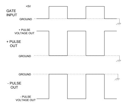
**Output Pulse Configuration With Inverted Gate Selected**
