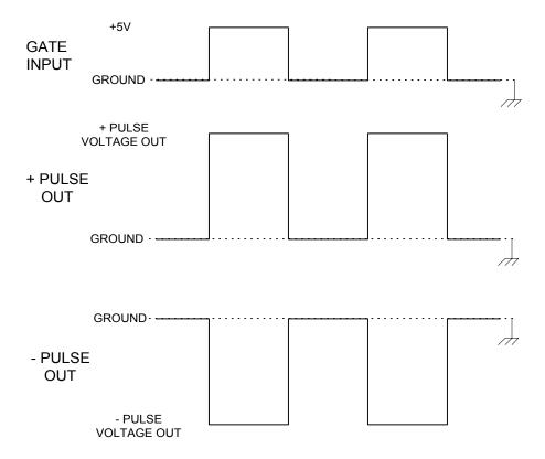
Output Pulse Configuration With Non-Inverted Gate Selected
