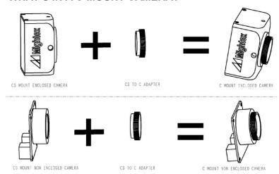
A C-mount camera is composed of a CS-mount camera and a CS-to-C-mount adapter. The latter is essentially a 5mm thick threaded ring.
