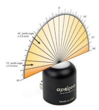
Directional, or cosine, response is defined as the measurement error at a specific angle of radiation incidence. Error for Apogee S2 series PAR-FAR sensors is approximately  $\pm$  2 % and  $\pm$  5 % at solar zenith angles of 45° and 75°, respectively.
