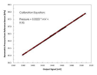
Example of SB-100 barometric pressure sensor calibration. Barometric pressure measurements from a reference sensor are plotted against the output signal voltage from the SB-100. A linear equation fitted to the data yields the calibration factor and offset, 0.0222 and 9.93, respectively, for this example.
