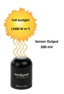
Example of total shortwave radiation measurement with an Apogee SP-110 pyranometer. Full sunlight yields total shortwave radiation on a horizontal plane at the Earth's surface of approximately 1000 W m<sup>-2</sup>. This yields an output signal of 200 mV. The signal is converted to shortwave radiation by multiplying by the calibration factor of 5.0 W m<sup>-2</sup> per mV.
