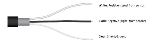
Wiring for SP-110 Serial Numbers range 0-60050
