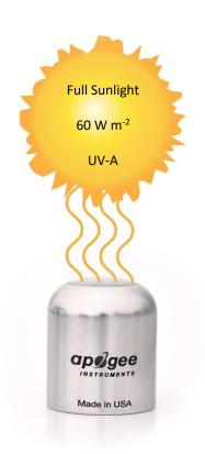
Example of UV-A measurement with an Apogee SU-202 sensor. Full sunlight yields UV-A radiation on a horizontal plane at the Earth's surface of approximately 60 W m $^{-2}$ . This yields an output signal of 1500 mV. The signal is converted to UV-A radiation by multiplying by the calibration factor of 0.04 W m $^{-2}$  per mV.
