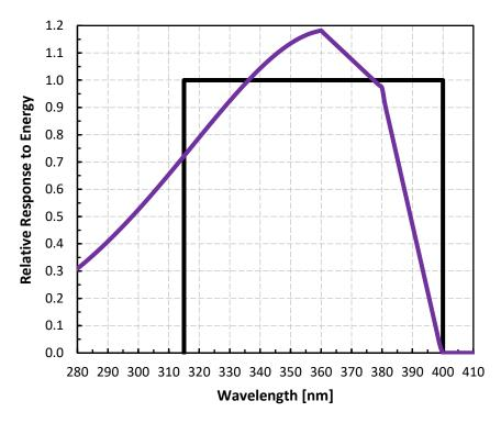
Spectral response estimate of Apogee SU-200 UV-A sensors. Spectral response was modeled from sensitivity of the photodetector and transmittance of the diffuser.
