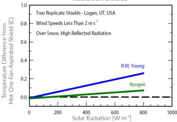
The performance of Apogee (model TS-100) and R.M. Young (model 43502) fan-aspirated shields relative to a Met One (model 076B) fan-aspirated shield.
