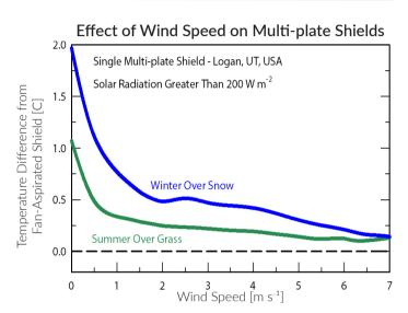
Naturally aspirated shields are subject to significant measurement errors when wind speeds are less than 3 ms<sup>-1</sup>. Errors increase when snow covers ground surface.
