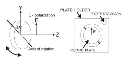
3. Rotate the screw, until the required retardation is achieved.
