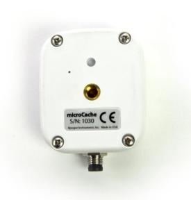
A sensor's model number and serial number are located on the back of the  $\mu$ Cache unit. If you need the manufacturing date of your  $\mu$ Cache, please contact Apogee Instruments with the serial number of your  $\mu$ Cache.
