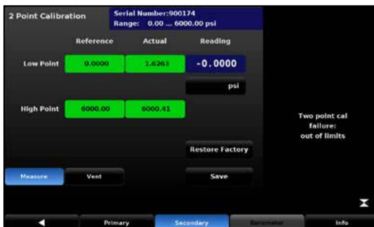
Figure 6.4.2.5.2-9 – ‘2 Point Calibration Failure’]
