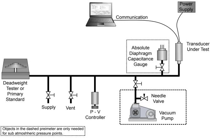
Figure 7.2.5 - Calibration Setup
